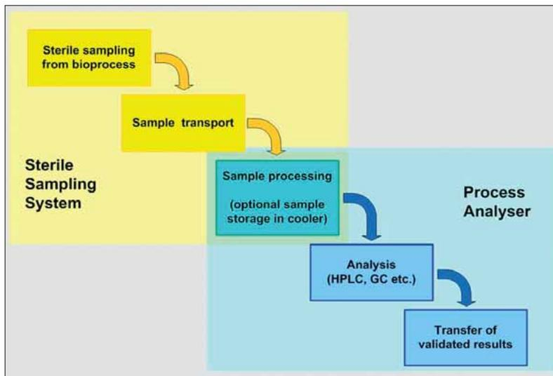
**Fig. 1: Complete workflow for automated bioprocess monitoring with routine-lab-equipment. Reliable sterile sampling, sample transport and subsequent sample processing is a prerequisite for any further analysis. Finally, validated results are visualized and can be transferred to superior expert systems, where they serve as input values for soft-sensors and potential control loops.**
